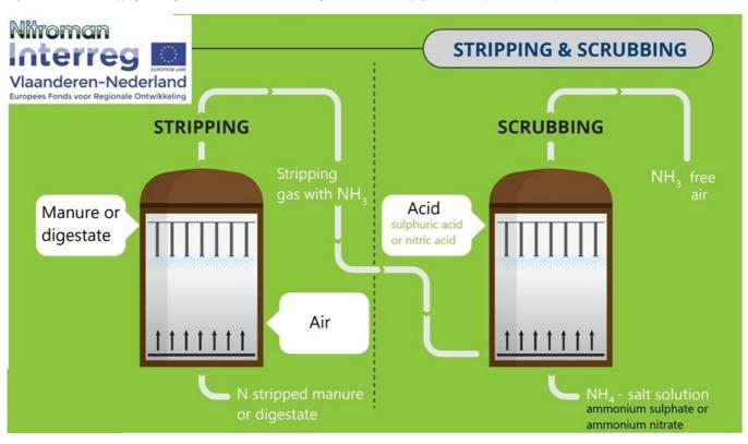
Adjusted scheme for NH3-stripping scubbing made in the framework of the Interreg Flanders-Netherlands project NITROMAN (www.nitroman.be)
