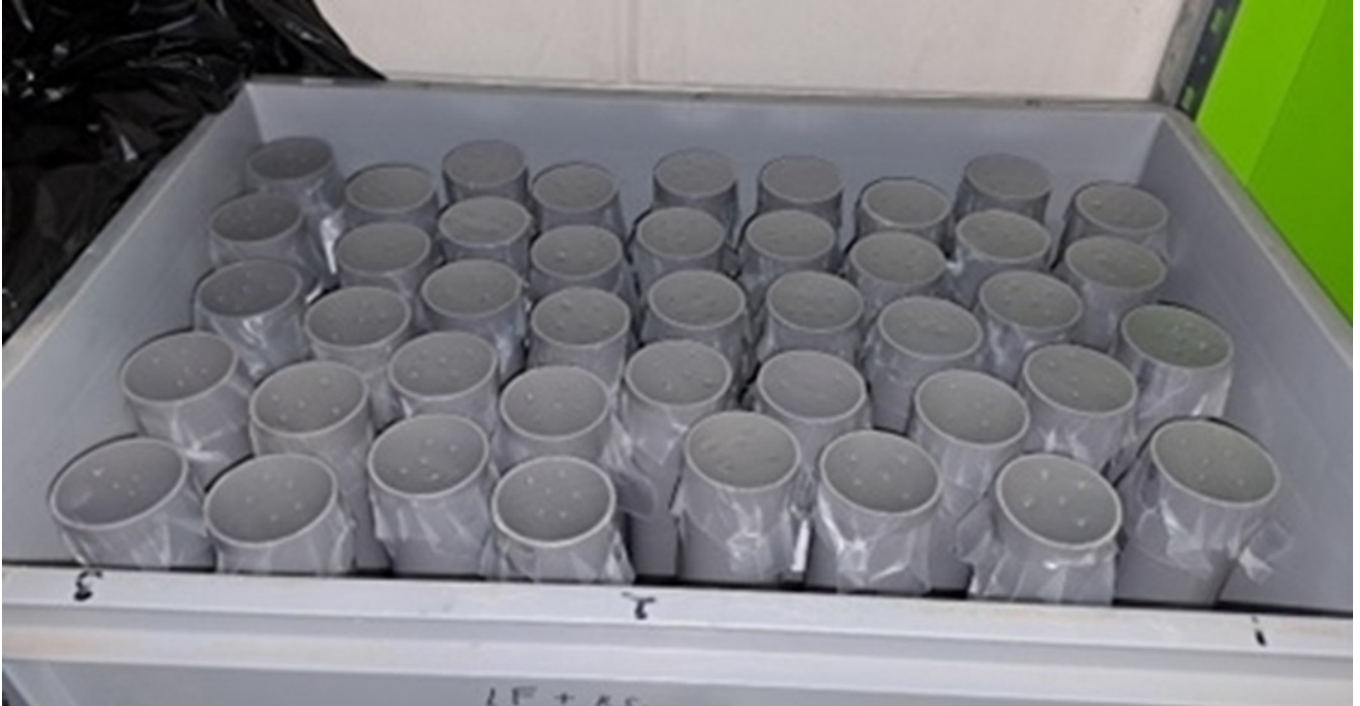
Figure 4: Tubes filled with soil and N-fertilisers in the soil incubation experiment ©Ghent University
