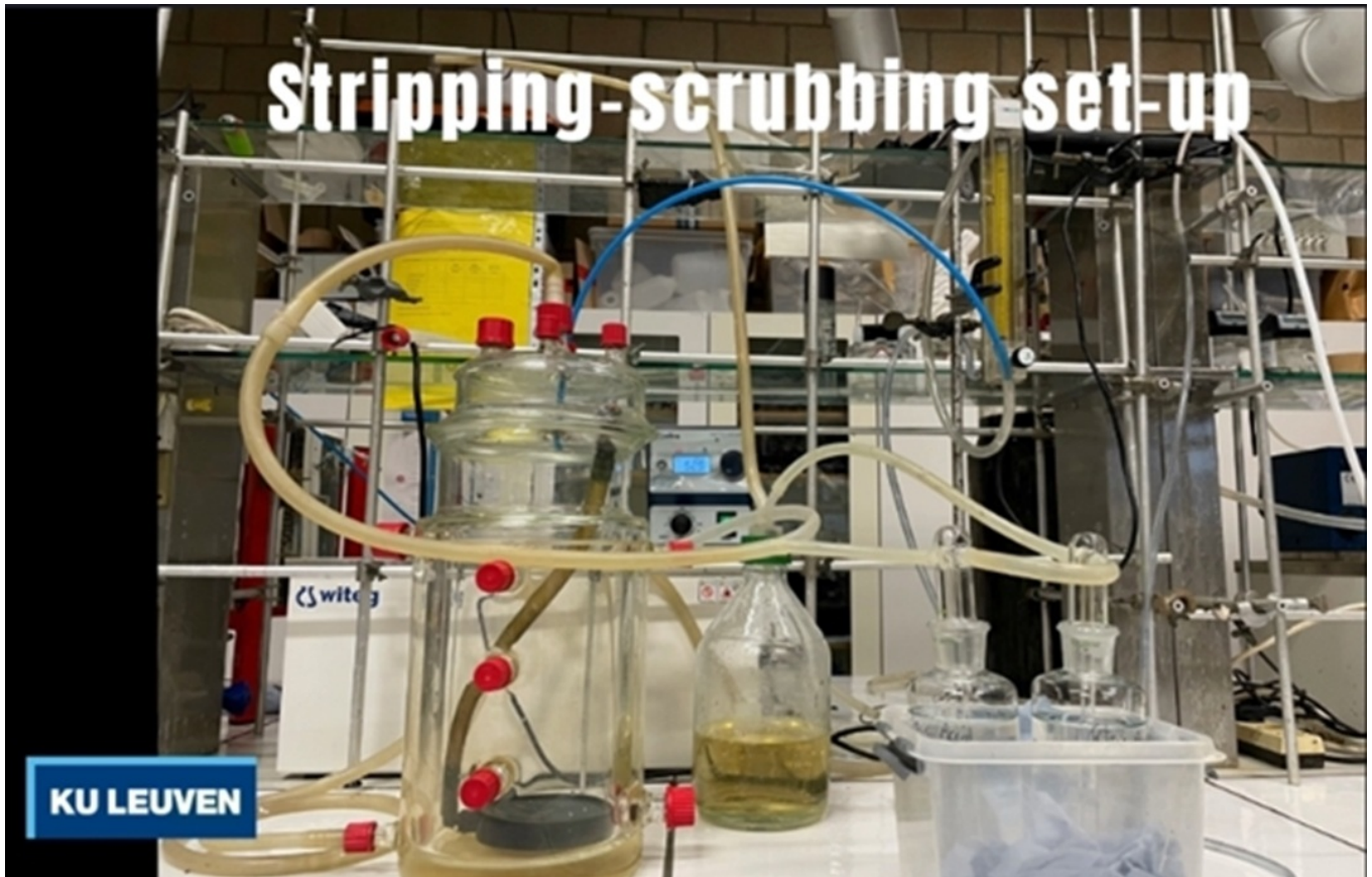
Figure 1: Stripping-scrubbing set-up, watch the experiment in action ©KU Leuven
